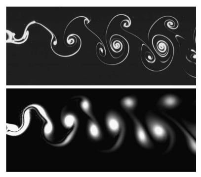
Fig. 7. Top: flow visualization of P + S wake pattern behind an oscillating cylinder at Re = 140 (C.H.K. Williamson, private communication). Bottom: gray scale plot of the vorticity field from a numerical simulation by Ponta and Aref (2006).
